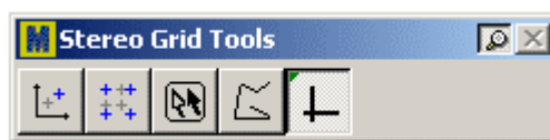
Figure 4: Stereo Grid Tools are used to adjust the size and/or position of the sampling grid.
