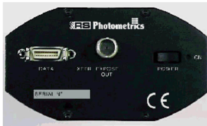
Figure 4: Rear view of CoolSNAP Color camera body.
